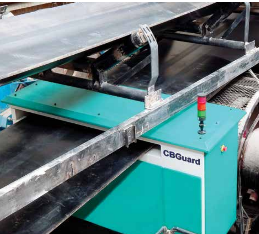
Left: CBGuard system in place on a conveyor.
